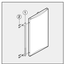
Secure handle 1 to the holes in the door using the screws marked 2.
